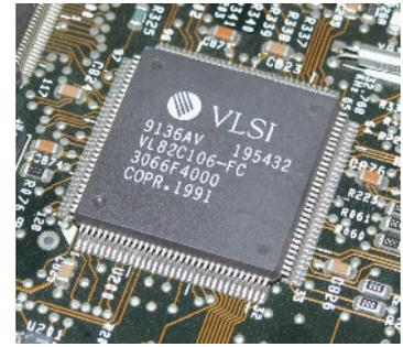
Fig. 1.11: VLSI chip
