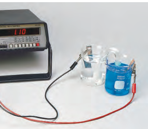
An electrochemical cell with a measured potential of 1.10 V.
