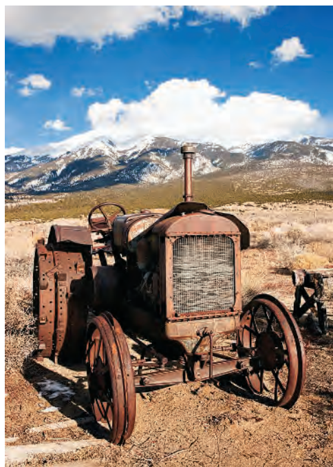
Formation of rust on bare steel is a spontaneous process.
