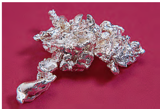
Crystalline silver contains cubic closest packed silver atoms.
