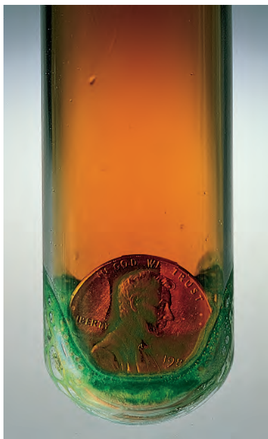
A copper penny reacts with nitric acid to produce \text{NO} gas, which is immediately oxidized in air to give reddish brown \text{NO}_2 .
