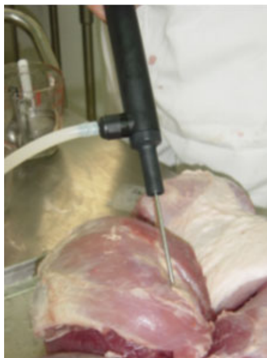
Fig. 226: Manual brine injection
