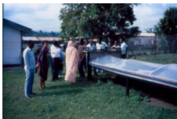
Fig. 291: Completed simple solar collector, covered with transparent UV resistant plastic sheet
