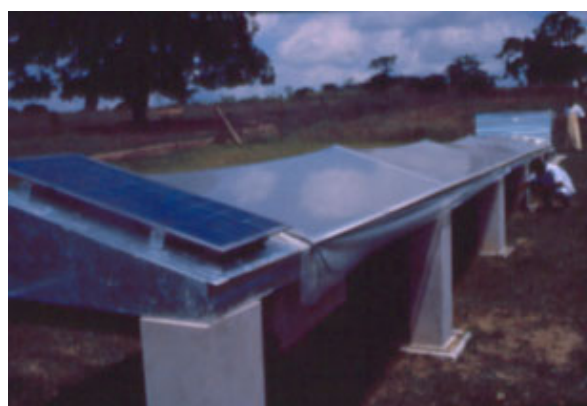
Fig. 293: Higher-cost construction of tunnel dryer. Roof-shaped solar collector, top part made of metal frames and bottom part made of metal-coated polyurethane panel. Length 15m. (Type 2 in table 13).
