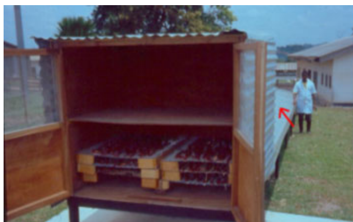
Fig. 294: Drying chamber (made of wood) connected to solar collector (arrow) of tunnel dryer. Trays with meat to be dried positioned in the chamber
