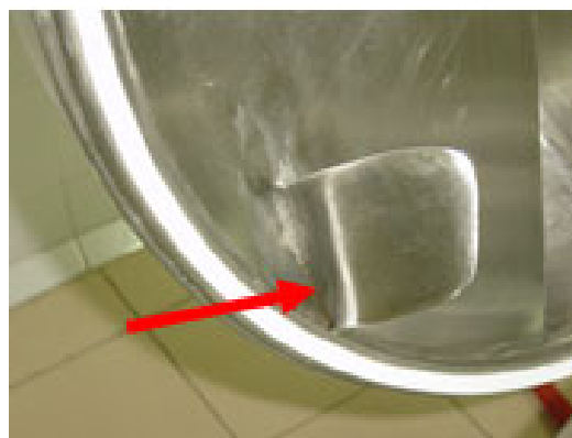
Fig. 400: Paddle on bowl cover with critical spot for cleaning
