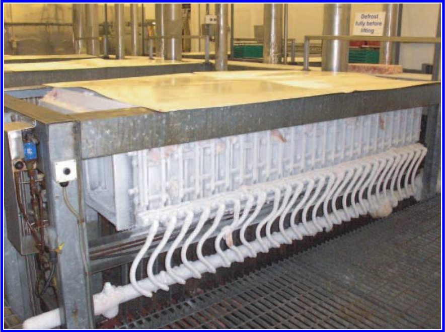
Fig. 23.2 Vertical plate freezer for freezing of blocks of boned meat.
