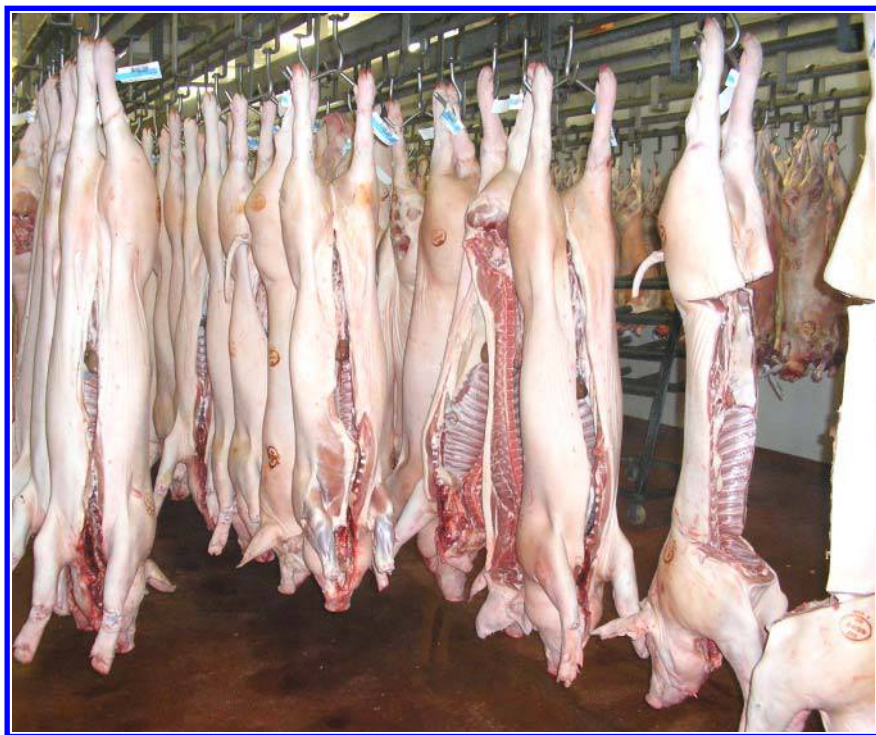
Fig. 23.1 Traditional primary air blast chilling of pig and lamb carcasses in a small multi-species abattoir.
