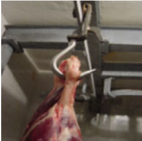
Fig. 481: Adequate material for refrigerated rooms: Overhead galvanized rails and beams, stainless steel meat hook
