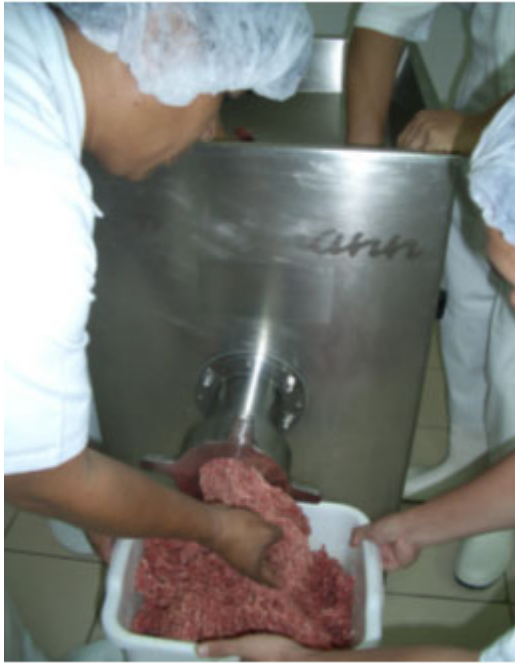
Step 2: Grinding/blending of burger mix
