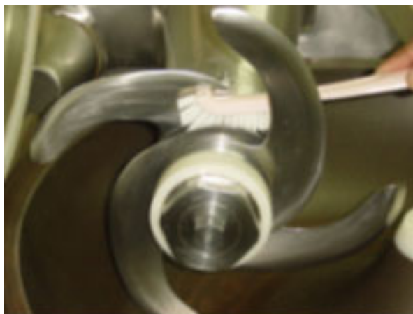
Fig. 399: Gap between bowl and knife shaft.
