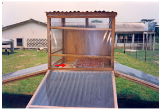
Fig. 296: Drying chamber of multi-collector dryer. Front and side walls of the chamber are transparent to collect additional solar energy. Air inlet from collector to chamber
