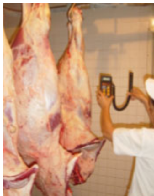
Fig. 426: Hygrometer. Measurement of rel. humidity in meat chiller
