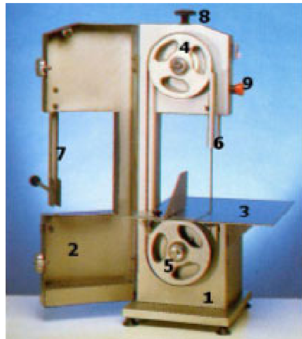
Fig. 404: Band saw open 4 – adjustable tensioning wheel 5 – drive wheel (connected to motor) 6 – band saw blade guide 8 – tensioning knob 9 – emergency switch
