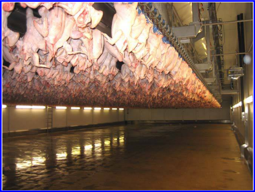
Fig. 23.5 Continuous air blast chilling of chicken carcasses.
