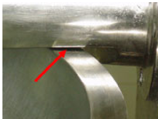
Fig. 399: Gap between bowl and knife shaft.
