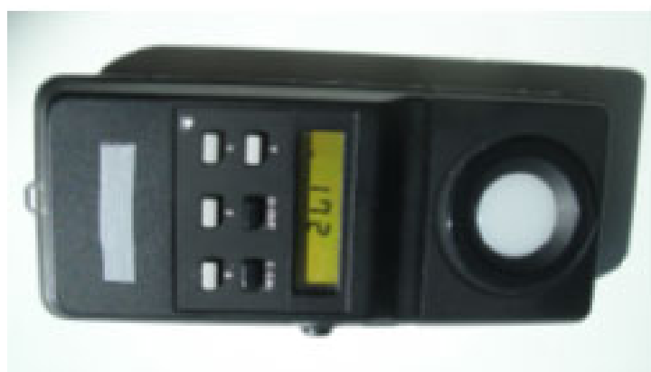
Fig. 431: Lux-meter Light sensor and monitoring unit in one portable instrument
