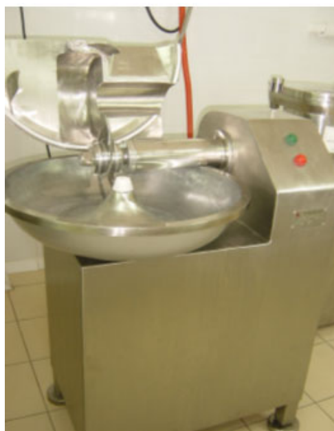
Fig. 312: Bowl cutter (18 litres) single phase power
