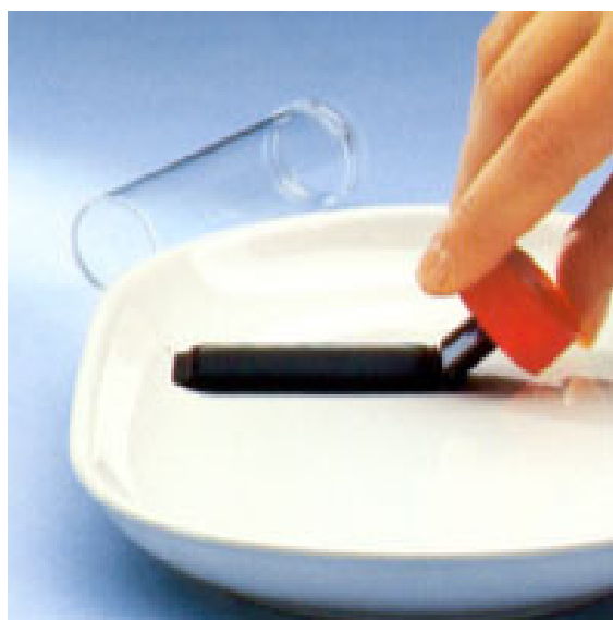
c) Test chip for contact method in action. Plastic tube (behind) to cover test chip upon use
