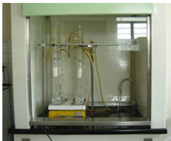
Fig. 436: Soxhlet extraction apparatus (for fat)
