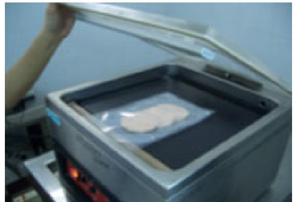
Fig. 344: Start of evacuation in vacuum packaging machine
