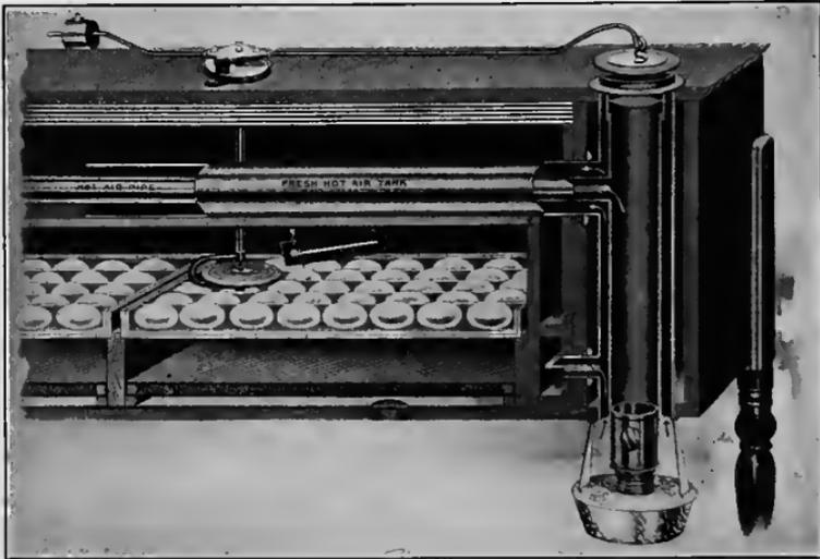
Hot-air incubator. Using both radiation and diffusion. (Courtesy of Sears, Roebuck & Company.)
