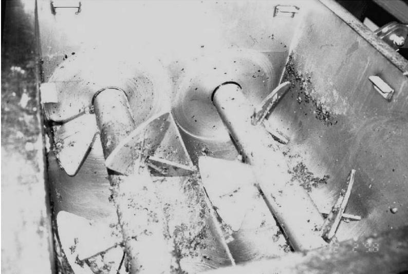
*Figure 12.1* View inside a mixer/blender showing the mixing paddles.
