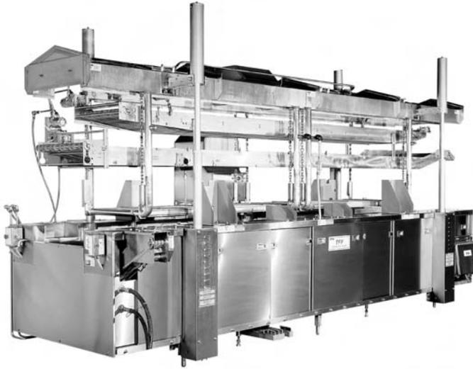
**Figure 15.10** Stein TFF-II Fryer, with top raised (Courtesy of Stein, Inc.)
