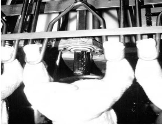
*Figure 3.14* Cropper showing serrated probe preparing to enter abdominal opening of the carcass.
