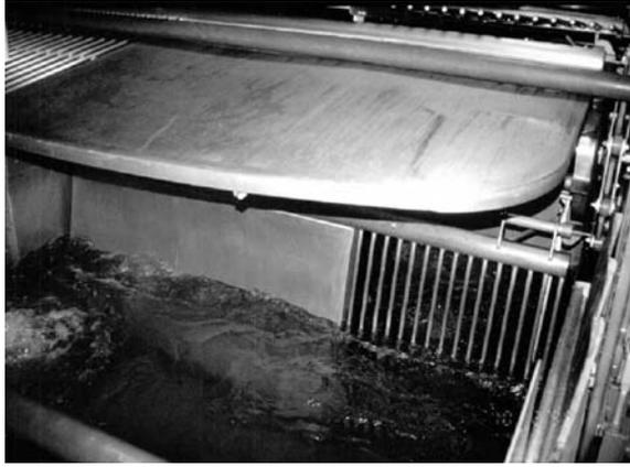
**Figure 3.16** Paddles in a chiller to move carcasses. Open side of paddle alternates between paddles to agitate the water.
