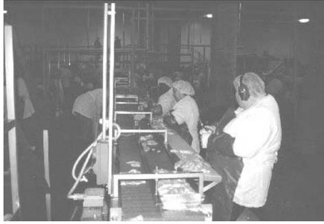
**Figure 4.5** Trimming and portion sizing line in plant producing boneless breast fillets.
