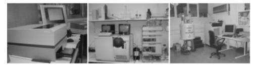
**Fig. 4.3** Advanced instruments used for laboratory quality control – ELISA reader, HPLC-MS/MS and NMR spectrometer (from left to right).
